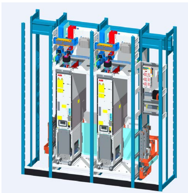
ACS880 retrofit for ACV700/SamiStar mechanical design with 2 modules.
