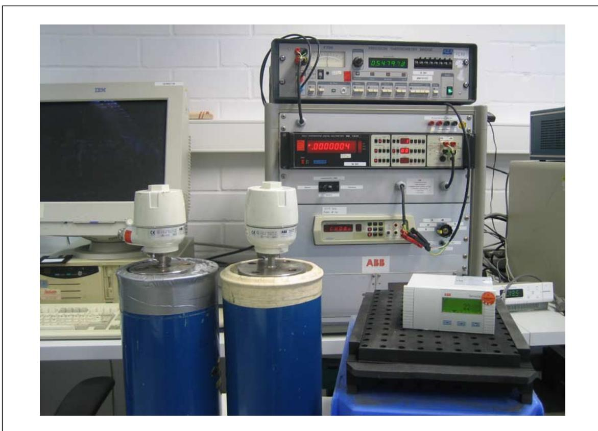
Fig. 2-1: Calibration setup of the measuring system
