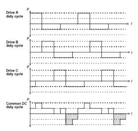
To define the load cycle of the system, you must first define the load cycle for each drive separately, and then calculate load cycle for the whole system based on the definitions and formulas given in the following sections.
