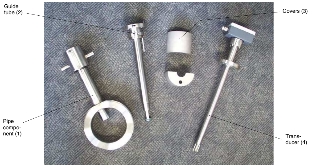
Fig. 4-11 Components of the integrated hot tap fitting
