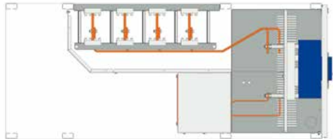
View from the top of a column with segregated moulded-case circuit-breaker in form 4b
