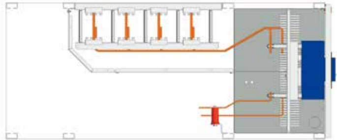
View from the top of a column with segregated moulded-case circuit-breaker in form 3b
