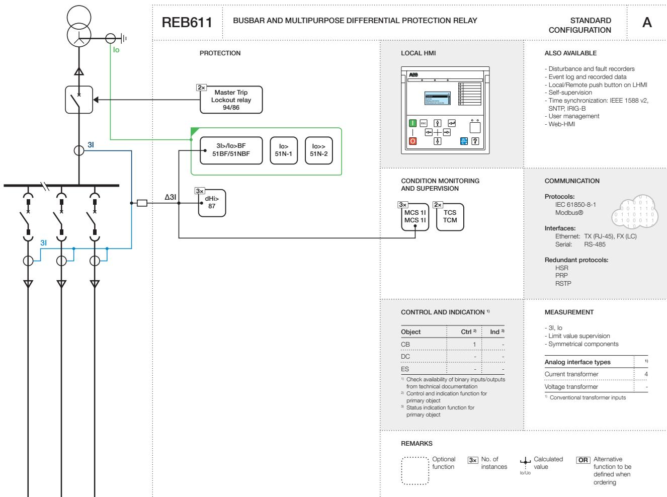
Figure 15: Functionality overview for configuration A
