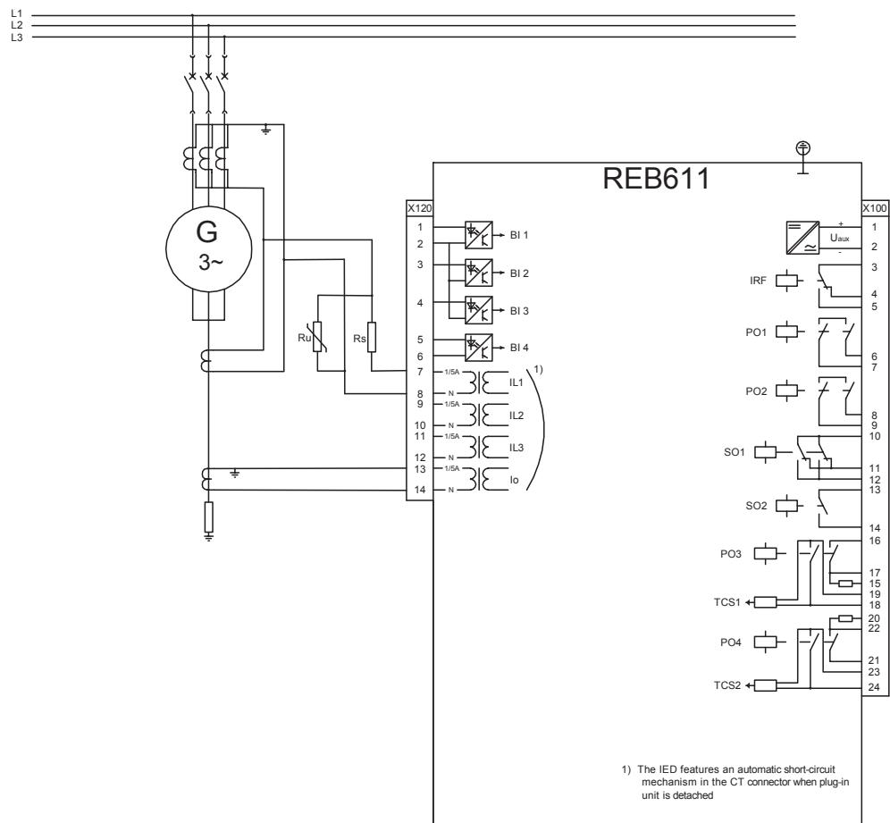
*Figure 14: Connection diagram for configuration A when used as rotating machine restricted earth-fault protection*
