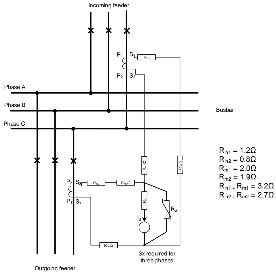
Figure 54: High-impedance busbar differential protection with different CT burden value on each feeder
