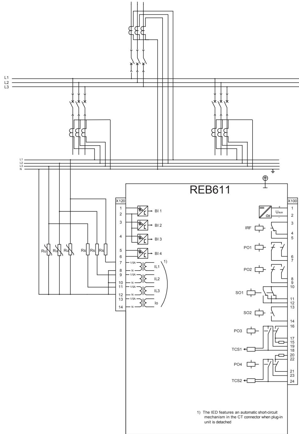
Figure 12: Connection diagram for configuration A when used as busbar differential protection
