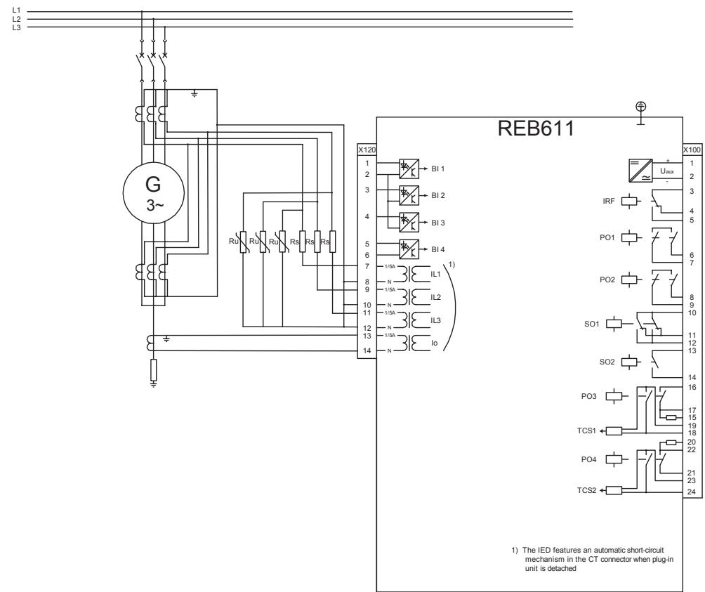
Figure 13: Connection diagram for configuration A when used as rotating machine phase differential protection
