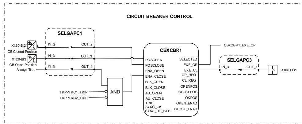
*Figure 23: Circuit breaker control*
