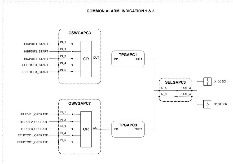
*Figure 24: Common alarm indication*
