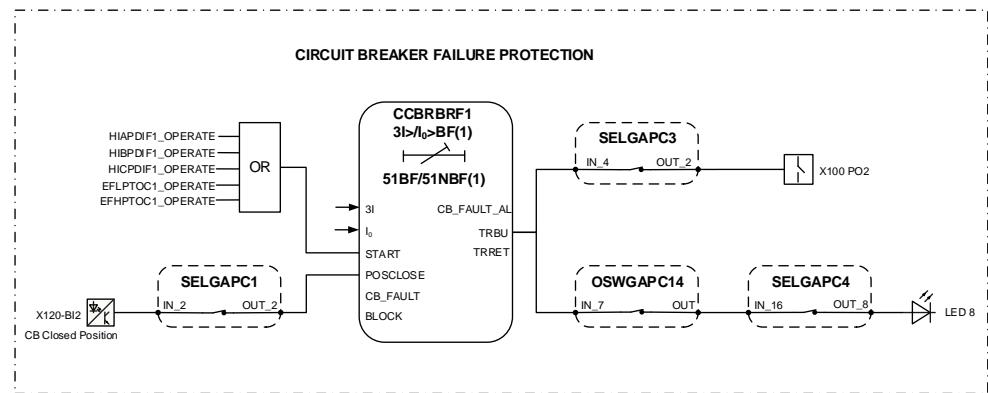
Figure 19: Circuit breaker failure protection
