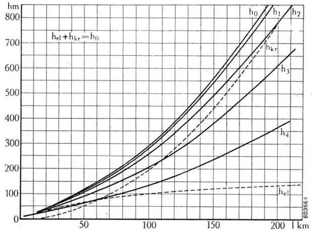
Fig. 3. — Necessary free heights for decimetre transmission.
