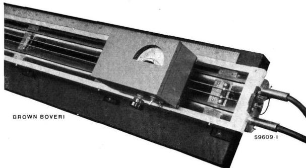
Fig. 1. — Parallel wire system for impedance measurements.
