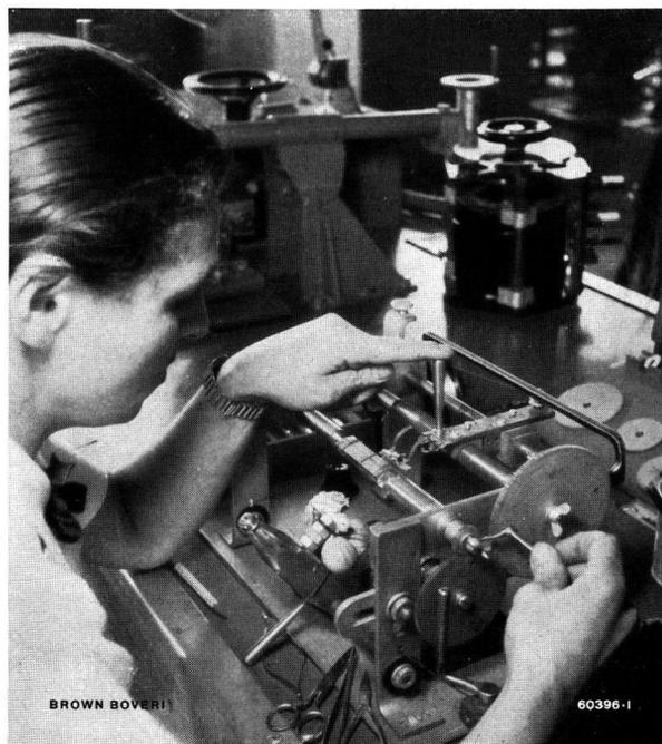
Fig. 2. — Grid winding machine.
