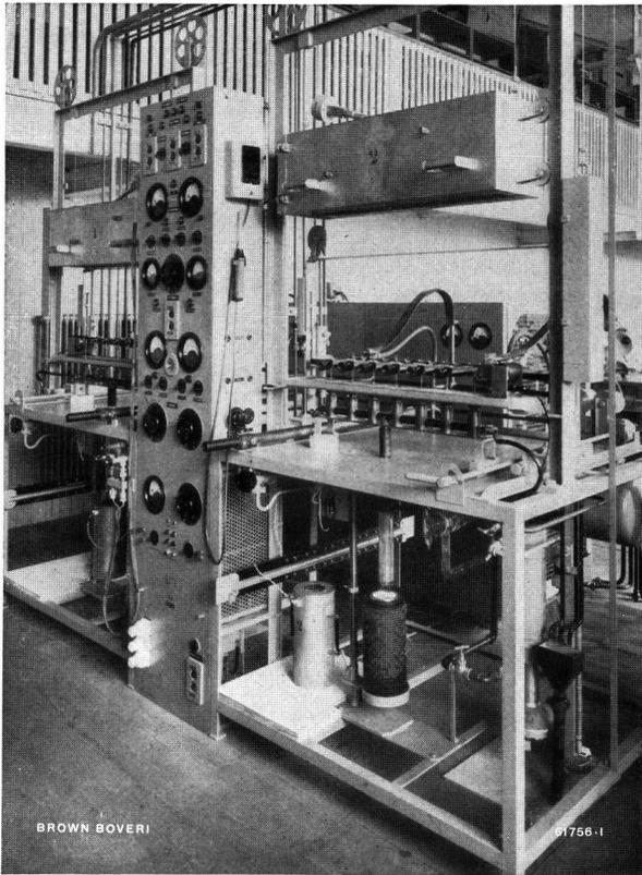
Fig. 3. — Double pump stand for small tubes.
