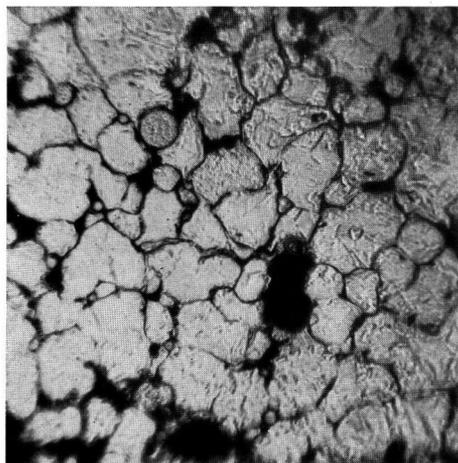
Fig. 2. — Metallograph of ground-surface specimen of an annular core. The iron powder referred to in Fig. 1 is moulded under high pressure. As a result the particles become heavily deformed, but the layer of insulation around them remains unimpaired. Permeability  $\mu = 40$ .
