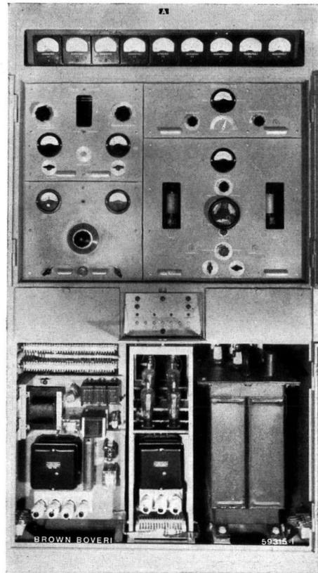
Fig. 9. — High-frequency preliminary stage of medium wave transmitter.
