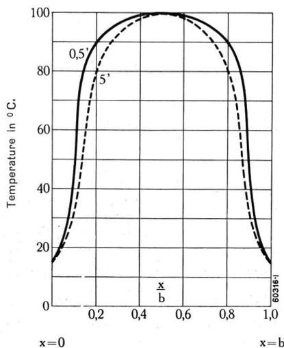
Fig. 2. — Temperature distribution through a laminated sheet heated with high-frequency power, after 0.5 and 5 minutes, respectively.
