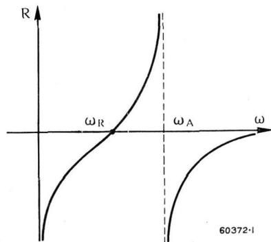
Fig. 7. — Reactance characteristic of a piezo-electric crystal in the vicinity of the fundamental resonance frequency.
