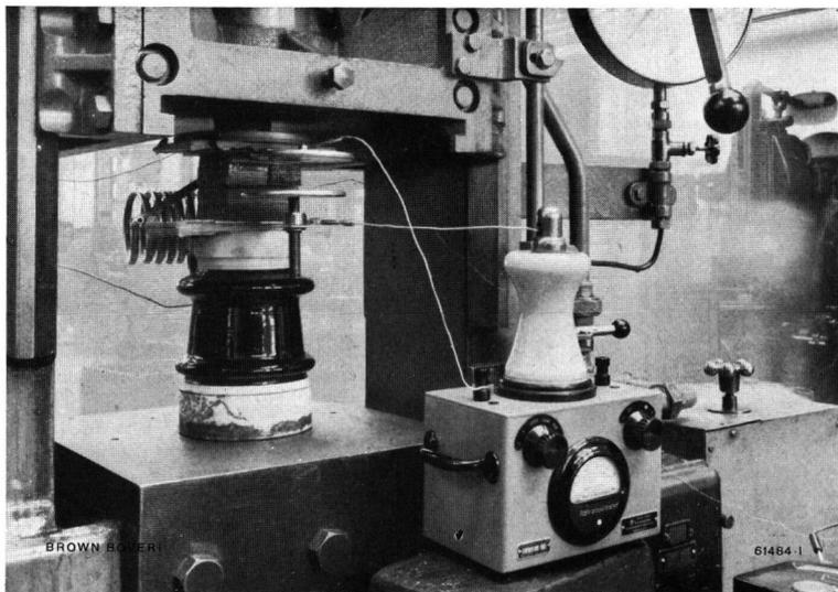
Fig. 5. — Test set-up for hardening laminated materials (compressed laminated wood) in a 20 t press.
