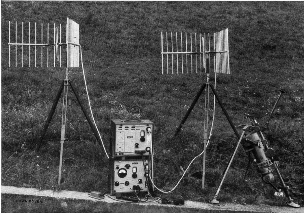
Fig. 5. — Complete beam station with frequency modulation for two-way communication over distances up to 200 km.
