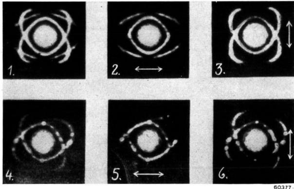
Fig. 2. — Diffraction of quartz in the  $x$  and  $y$  axes in unpolarized (1 and 4) and linear polarized light (2, 3, 5, and 6), according to Bergmann-Schäfer.
