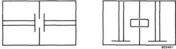
Fig. 7. — Cavity resonator band filters.
