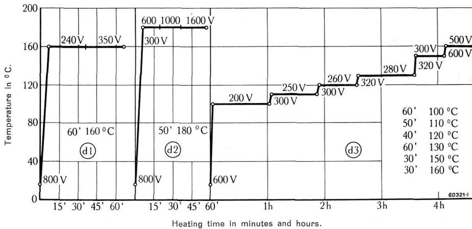
Fig. 8. — Characteristics of three different hardening conditions employed during tests, in relation to time, temperature, and voltage. In order to obtain comparable results these hardening conditions were employed both for stove and high-frequency heating.
