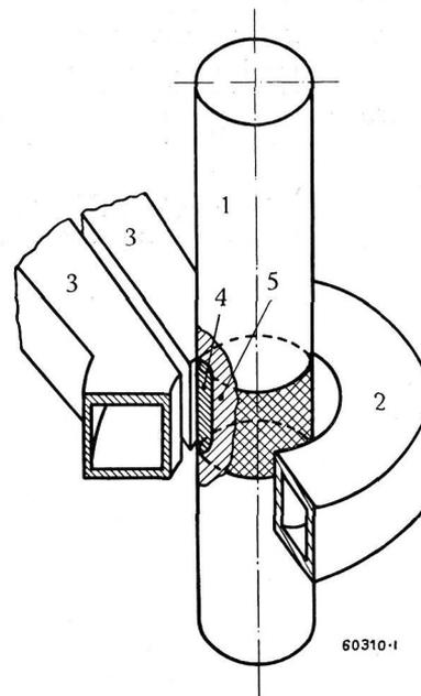
Fig. 3. — Diagram of arrangement of inductor and shaft for the surface hardening of various annular zones.
