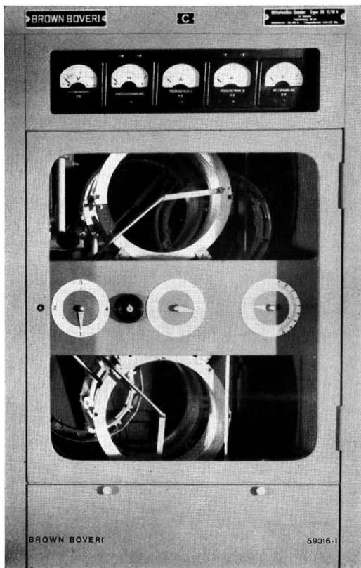
Fig. 10. — Coil panel of high-frequency output stage of medium-wave transmitter.
