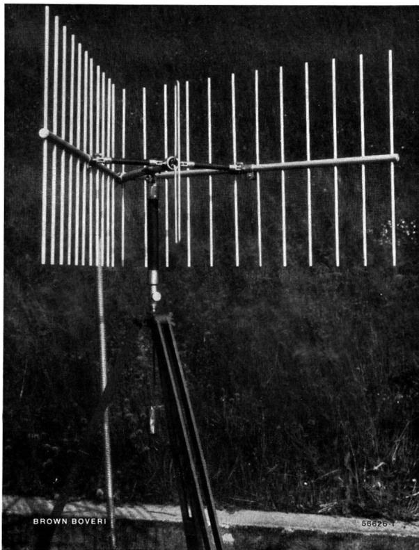
Fig. 1. — Directional antenna for very short radio waves. This simple antenna results in a tenfold increase in power in the desired direction when compared with a non-directional antenna.
