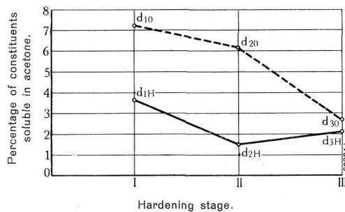
Fig. 11. — Percentage of pure phenolic resins soluble in acetone in various hardening stages.
