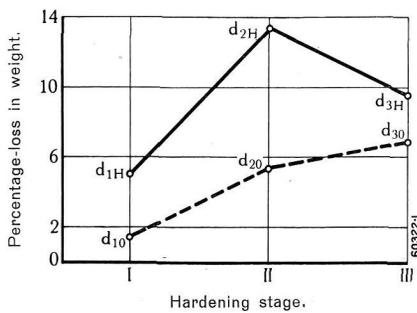
Fig. 9. — Relation between hardening losses of pure phenolic resins and hardening conditions shown in Fig. 8. Test series d.
