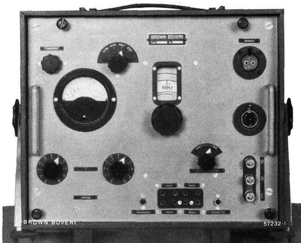
Fig. 6. — Directional receiver for the station shown in Fig. 5, in superheterodyne arrangement with limiter and discriminator, and four and two wire connections.
