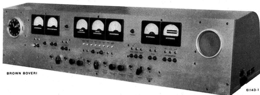
Fig. 4. — Control desk for short-wave transmitter.
