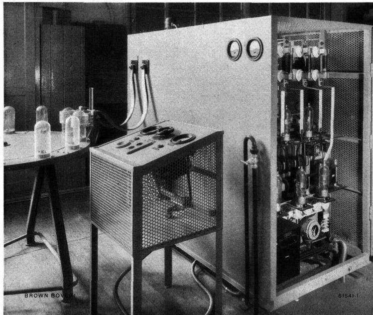
Fig. 1. — High-frequency generator for industrial purposes.
