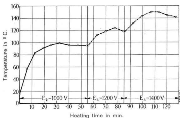
Fig. 6. — Relation between hardening temperature in laminated materials and voltage of high-frequency field.
