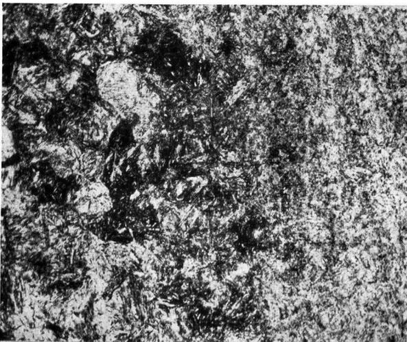
Fig. 5. — Microstructure of treated steel. Magnification 200 ×. On left, original material. On right, hardened material.
