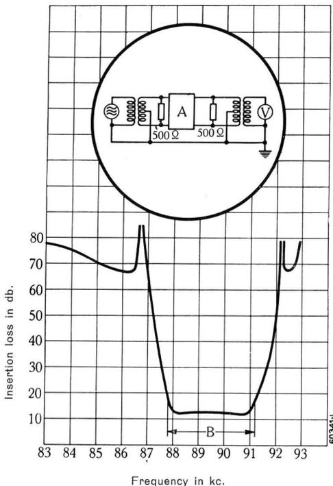
Fig. 12. — Measured insertion loss characteristic of crystal filter illustrated in Fig. 11.
