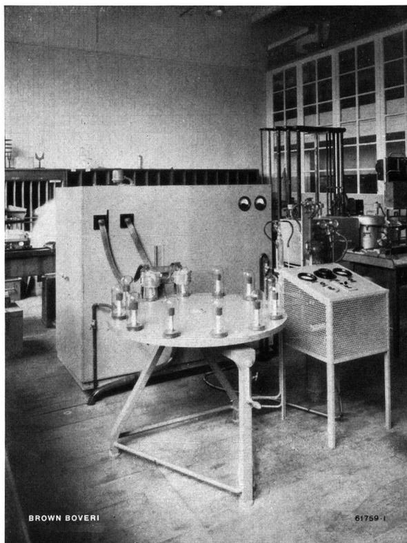
Fig. 1. — Socket sintering machine for manufacturing thin discs from glass powder and unglazed bushings.
