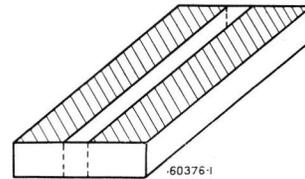
Fig. 13. — Crystal with divided electrodes.
