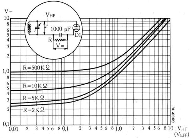
Figs. 5a and 5b. — Characteristics of diode D1.
