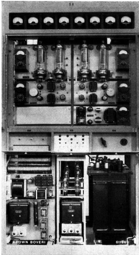
Fig. 8. — Low-frequency preliminary stage panel of short-wave transmitter.
