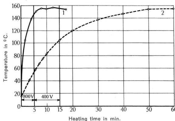
Fig. 7. — Comparison between temperature rise in pure phenolic resins in high-frequency field and in electrically-heated stove.
