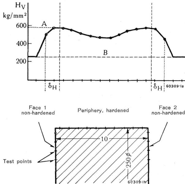
Fig. 2. — Measured hardness values of a chromium-steel disc in Vickers units.
