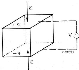
Fig. 1. — Schematic representation of polarization of a piezo-electric crystal under the effect of a mechanical force.
