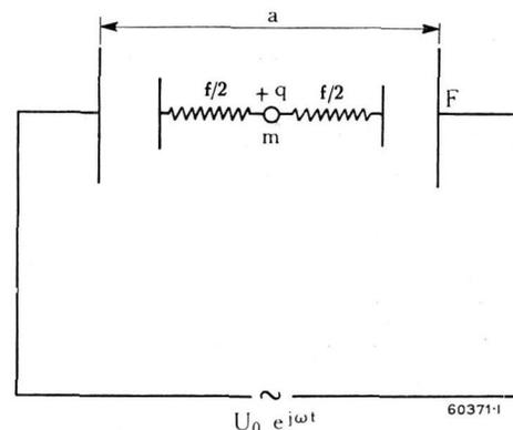
Fig. 6. — Mechanical model of a piezo-electric crystal.
