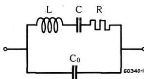
Fig. 5. — Equivalent network of a piezo-electric crystal oscillator.
