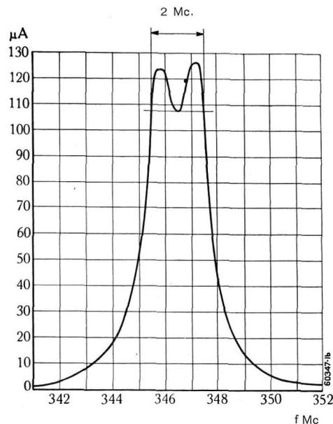
Figs. 8 and 9. — Measured band filter curves with inductively coupled cavity resonators for decimetre waves.
