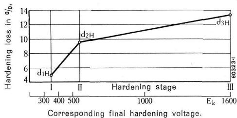
Fig. 10. — Relation between hardening losses of pure phenolic resins and applied voltage.
