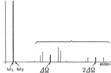
Fig. 1. — Frequency spectrum of output voltage of a f. m. detector with two f. m. voltages of slightly different frequency at the input.
