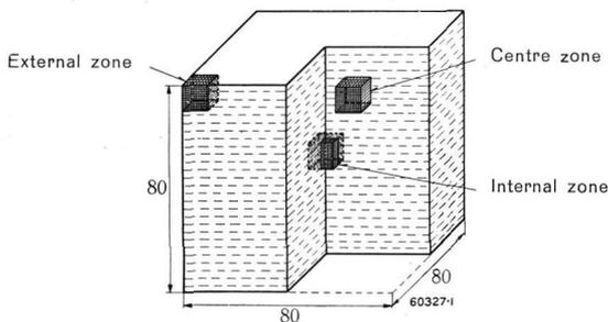
Fig. 13. — Points from which specimens of compressed laminated wood taken for tests.
