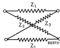
Fig. 8. — Schematic representation of a lattice filter.  $Z_1$  and  $Z_2$  are each two identical impedances in the series and diagonal arms.
