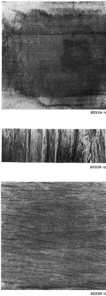
Fig. 15. — Effect of incorrect temperature characteristic (too rapid voltage rise at beginning of hardening process) on compressed laminated wood with heating by high-frequency power.
