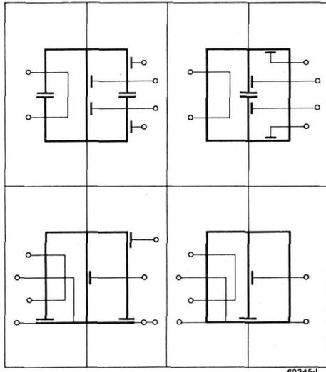
Fig. 6. — Cavity resonator couplings.
