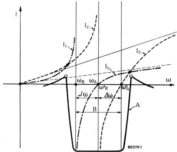
Fig. 10. — Attenuation characteristic of filter.
