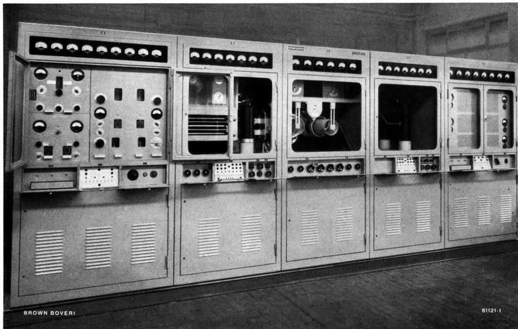
Fig. 2. — 10 kW short-wave transmitter type SO 25/10 k after acceptance in factory.
