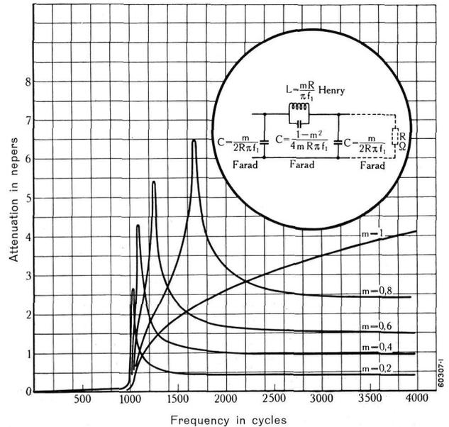
Fig. 3. — Computed attenuation curves for low-pass filters.
