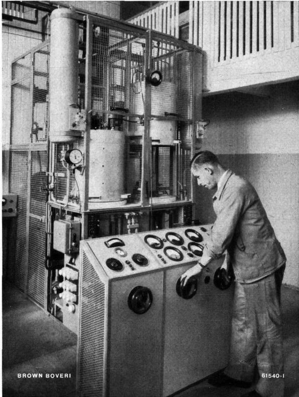
Fig. 2. — Pump stand for high-power transmitting tubes.
