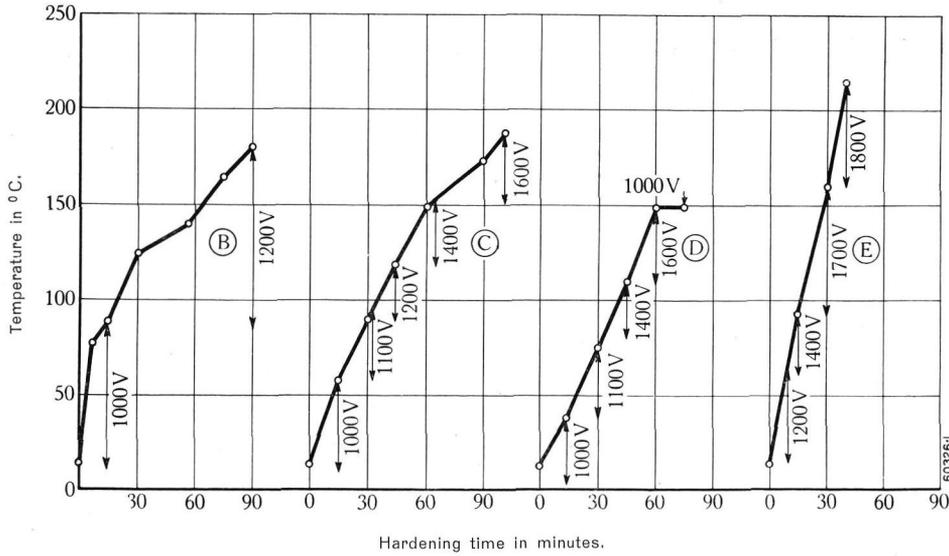
Fig. 12. — Characteristics of hardening conditions of compressed laminated wood investigated, in relation to temperature, time, and voltage.
