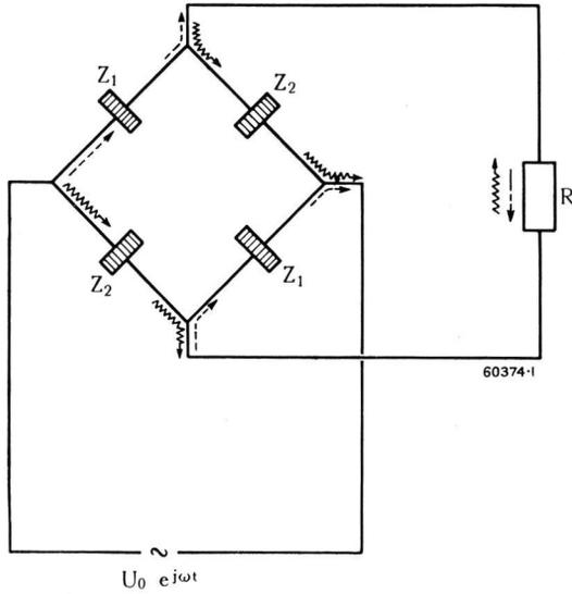
Fig. 9. — Simplified diagram of a bridge filter.
