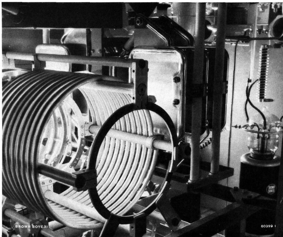
High-frequency output coil for a 10 kW broadcasting transmitter.
