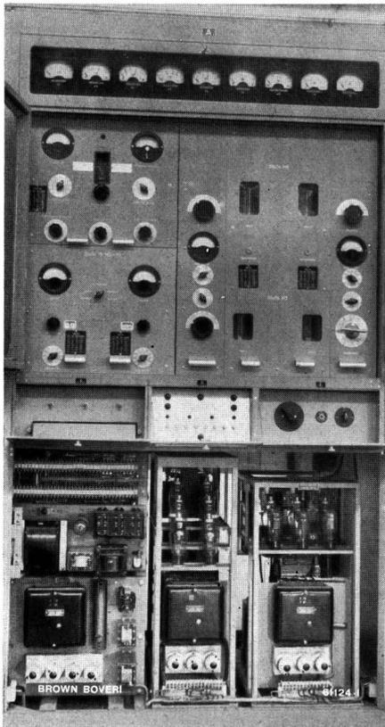
Fig. 5. — High-frequency preliminary stage panel of short-wave transmitter with door open.
