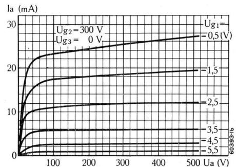
Figs. 7a and 7b. — Characteristics of pentode P2.
