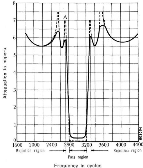
Fig. 2.— Attenuation characteristic (working attenuation) of band-pass filter with coils having Brown Boveri powdered iron cores, depicted in Fig. 1.
