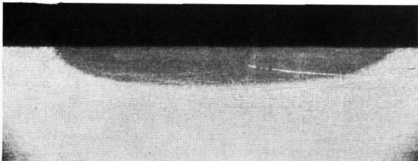
Fig. 4. — Surface ground specimen showing hardened zone 4. Magnification 10 ×.
