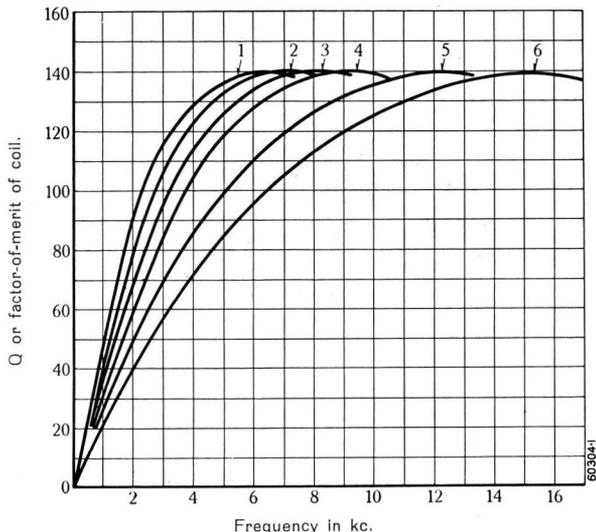
Fig. 3. — Factor-of-merit or Q of various annular types of cores.
