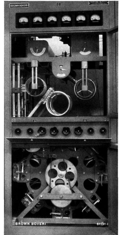
Fig. 7. — High-frequency output stage coil panel of short-wave transmitter.
