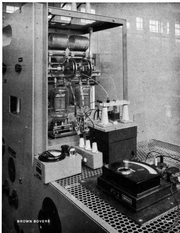
Fig. 4. — Test set-up for hardening of pure resins.
