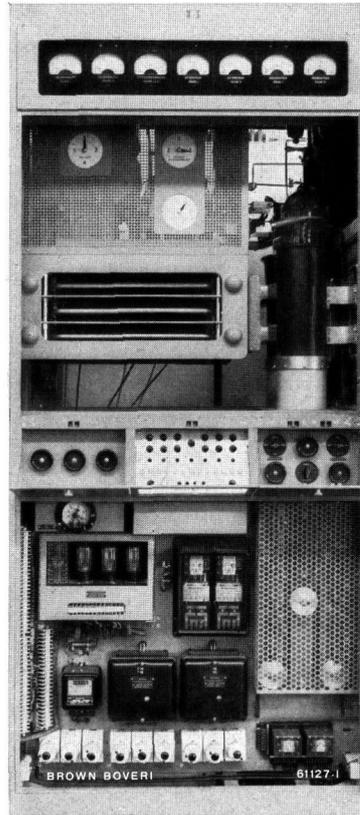
Fig. 6. — High-frequency output stage valve panel of short-wave transmitter.
