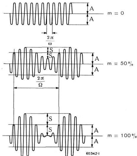
Fig. 1. — Amplitude modulation of a carrier wave by sinusoidal signals.
