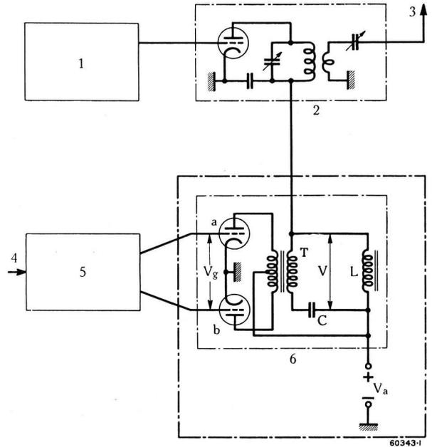
Fig. 2. — Theoretical circuit for anode modulation of a final transmitter stage by a class B modulator.
