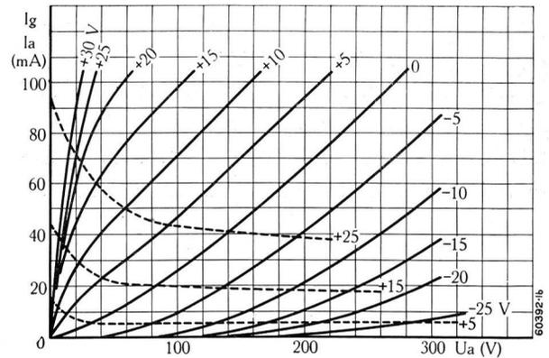
Figs. 6a and 6b. — Characteristics of triode T3.
