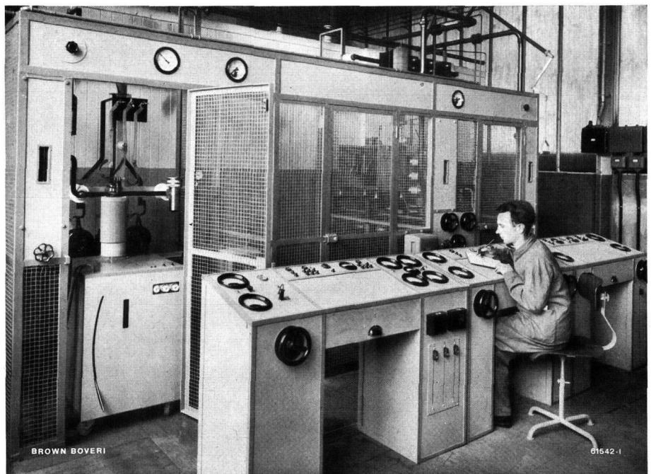
Fig. 3. — Test plant for the static and dynamic testing of high-power transmitting tubes.
