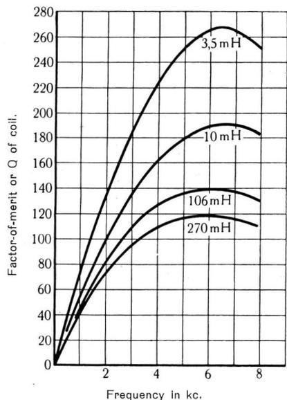
Fig. 4. — Factor-of-merit or Q for different numbers of turns.
