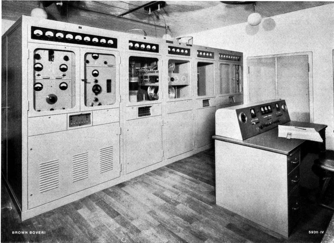
Fig. 1. — 10 kW medium-wave transmitter type SO 26/10 k, with control desk, ready assembled.
