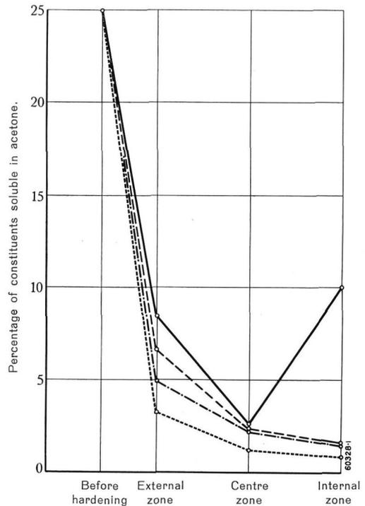
Fig. 14. — Percentage of constituents of various specimens soluble in acetone (internal, centre, and external zones).
