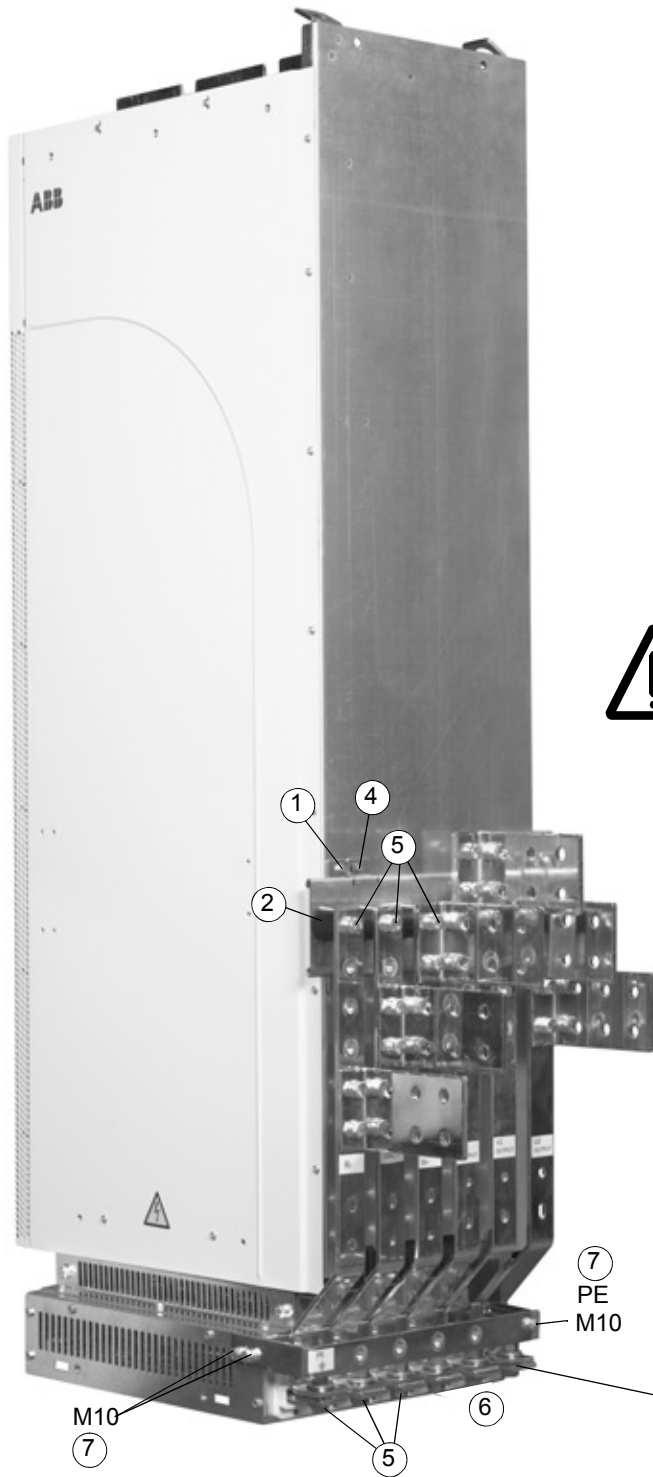
Frame size R8 +H360: AC, DC and brake busbars connected (+H356 included)
