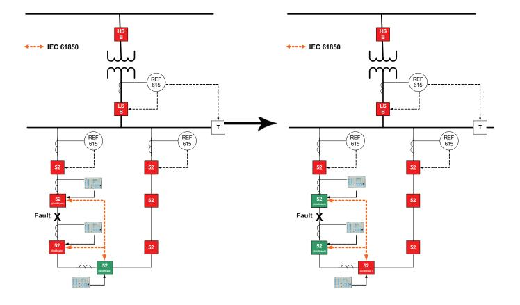
Figure 3. Recloser application with Distributed Energy Resources (DER)
