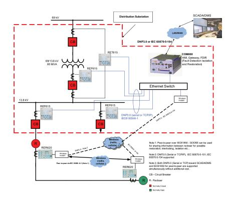
Figure 6. Industrial distribution network example using 615, 620 series protection and control relays, Station Automation COM600 and System 800xA
