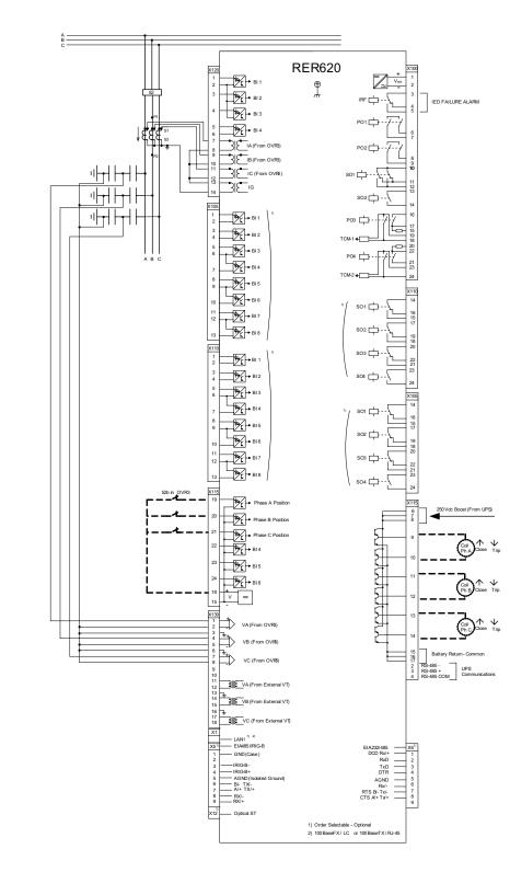
Figure 9. RER620 standard configuration A with options
