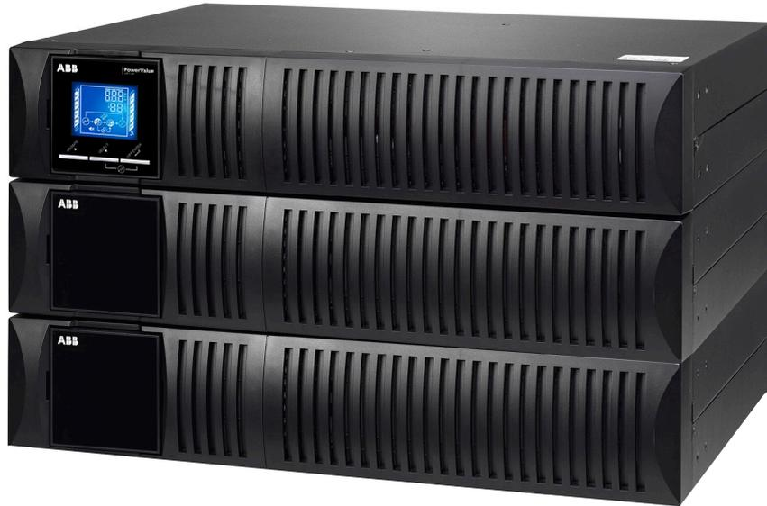
**Operation:** To recover the UPS's normal status, the EPO connector has to be set back to its original configuration (Normally closed through a jumper in the UPS rear panel). After this, the EPO status has to be cleared through the LCD menu and the UPS will recover its operation in bypass-mode. To transfer the UPS to inverter-mode, the selection has to be made through the LCD display.
