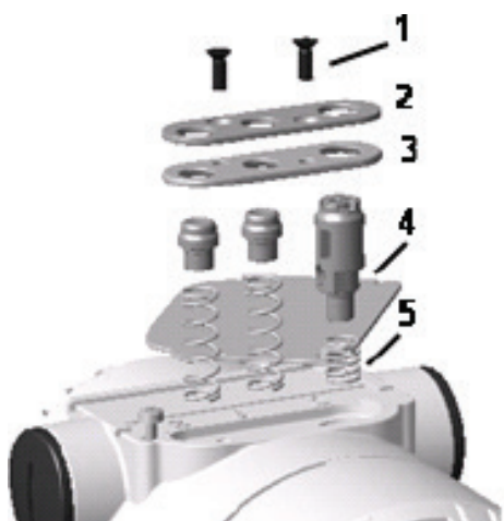
Figure 15 External push button assembly components
