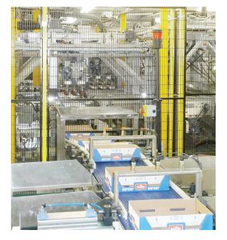
The functional requirement of the repack system was to take packed yogurt from a pallet, produce a multi pack, repack and palletise.
