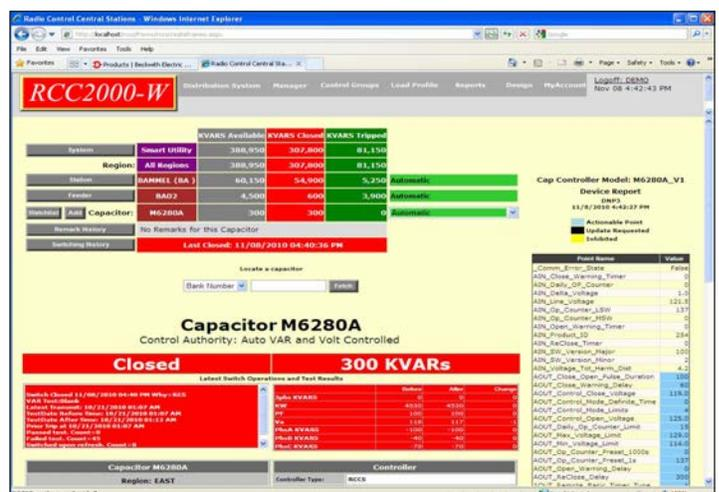
Figure 3 VVMS capacitor screen
