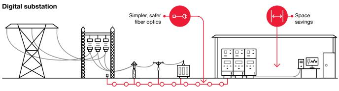
Smaller, safer and more efficient Digital substations replace many point-to-point copper cables with a single fiber optic process bus.
