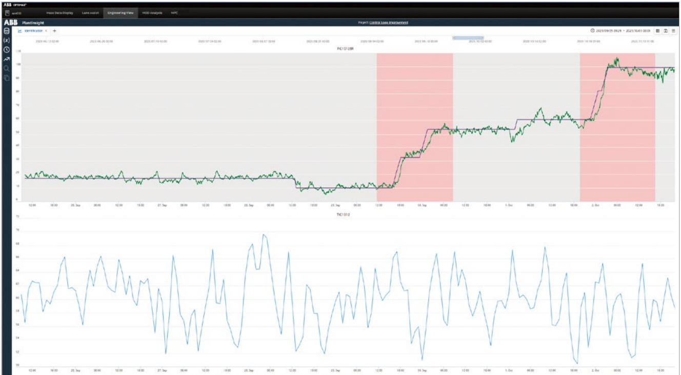
05 Example of automatically identified operating states that could be used for process identification. (gray = not-applicable, pink = applicable).
