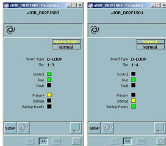
Figure 196. IOB Module (Primary) and Backup)
