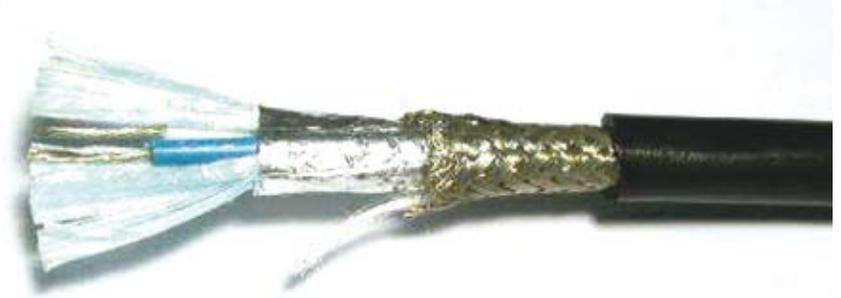
A suitable cable for this application is “BELDEN 82841” (nominal characteristic impedance 120 Ohms, nominal conductor DC resistance @ 20 °C 24 Ohms/1000 ft., max. recommend current 4 Amps per conductor @ 25 °C).
