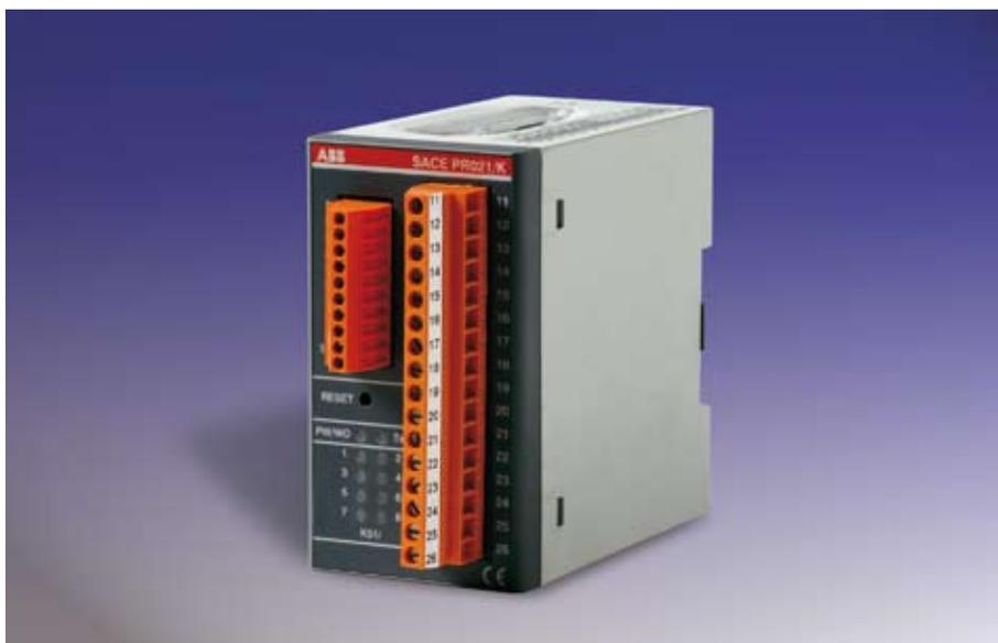
PR021/K signaling module converts the digital signals of the protection units into electrical signals via 8 normally open contacts.
