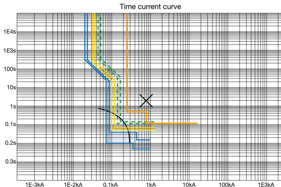
It can be noticed that total selectivity is guaranteed between X1 and T7 circuit-breakers through an effective setting of S protection.
