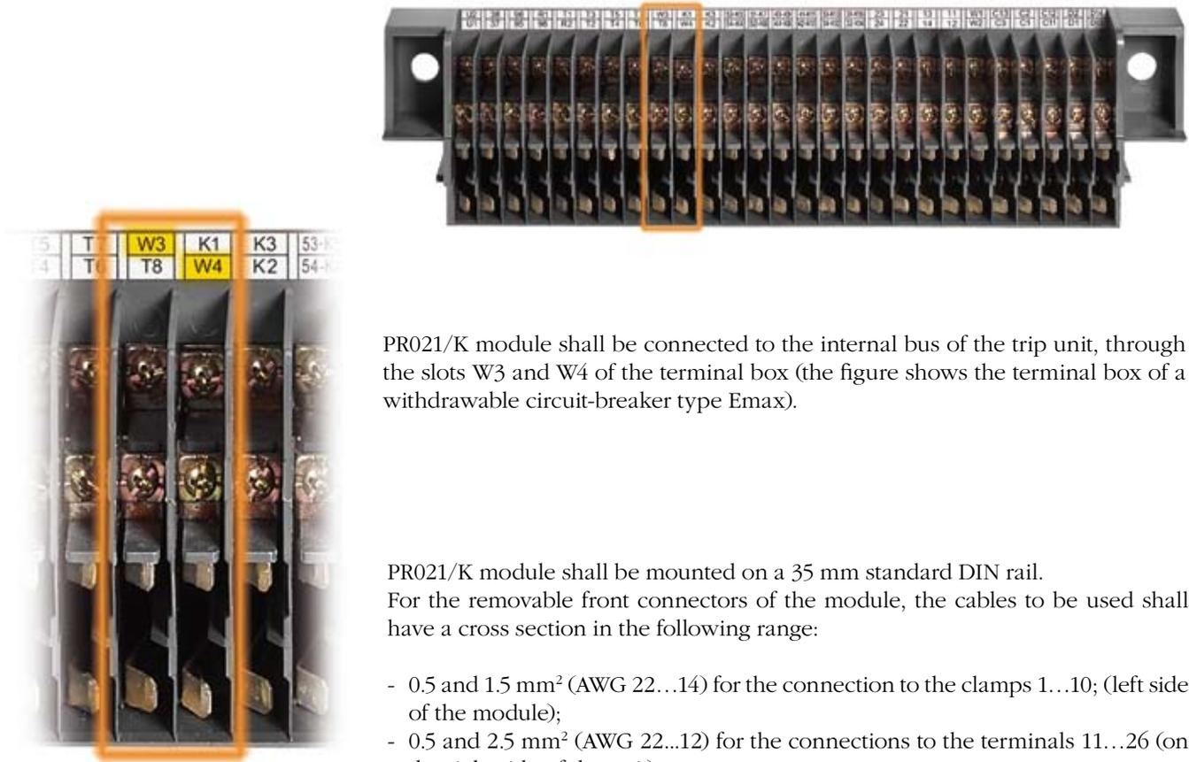
PR021/K module shall be connected to the internal bus of the trip unit, through the slots W3 and W4 of the terminal box (the figure shows the terminal box of a withdrawable circuit-breaker type Emax).
