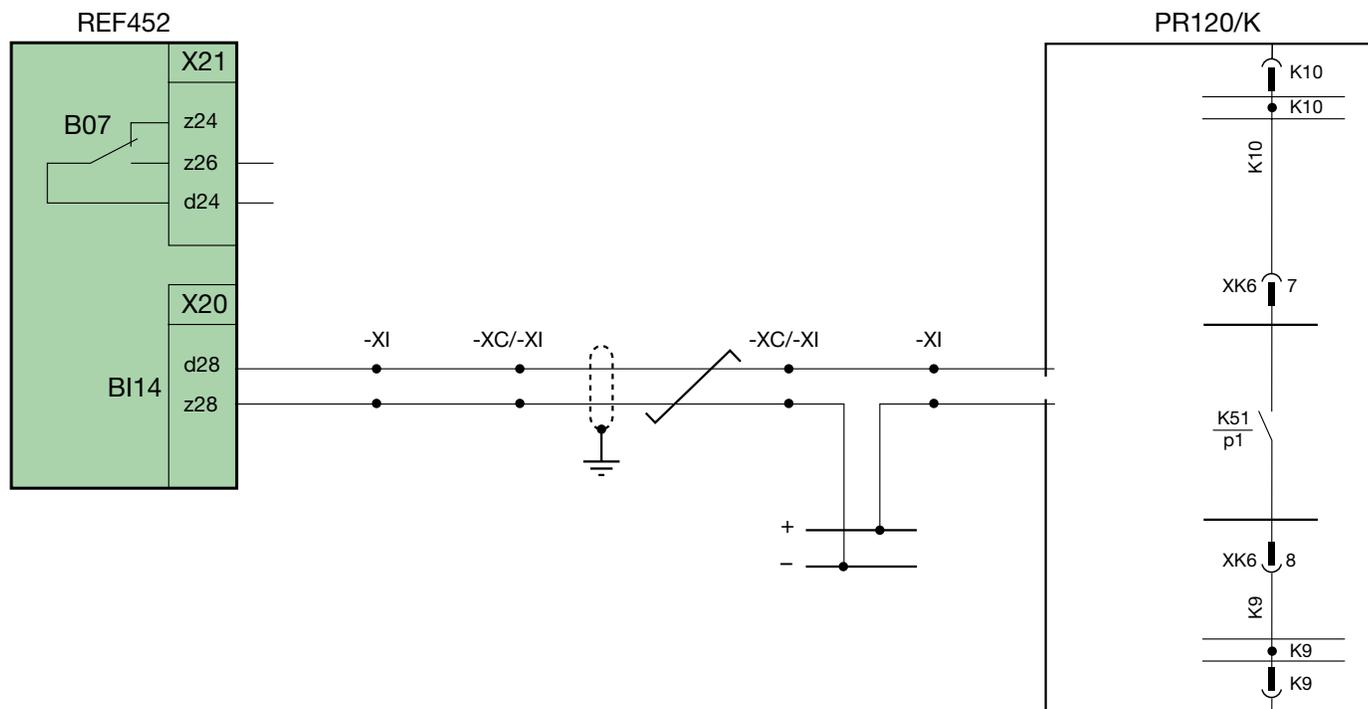
To set properly K51/p1 contact, it is possible to use the test and signaling unit PR010/T or the programs SD-Pocket (for PDA) or SD-TestBus (for PC); to send the block signal to the MV product, it is necessary that the contact K51/p1 is set as follows:
