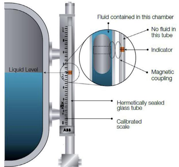
Figure 3 Magnetic Level Gauge Principle
