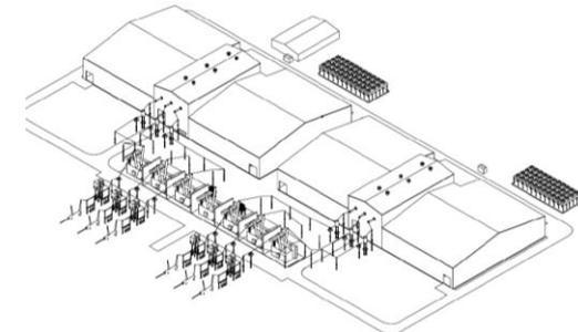
**3 x  $\pm 320$  kV HVDC Light tripole**
