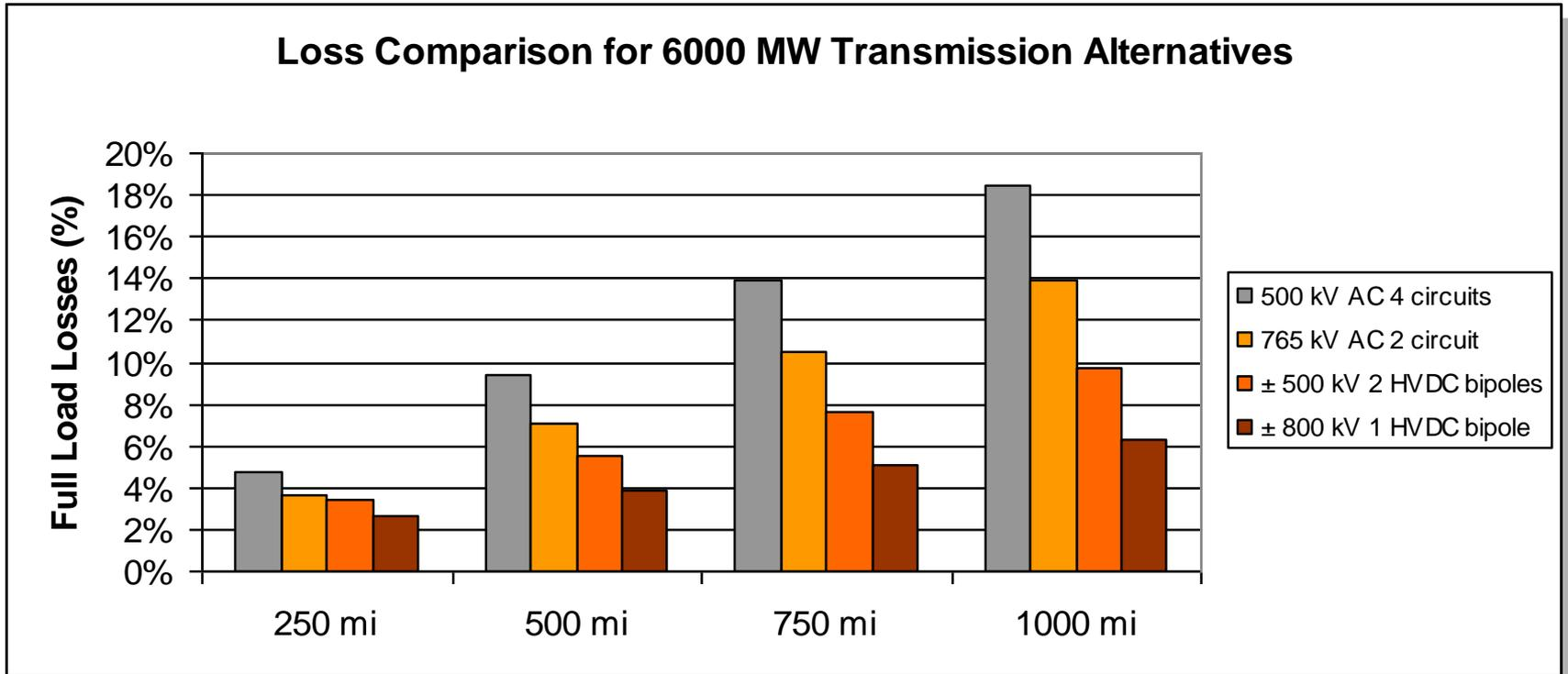
Note: AC and DC line conductors chosen for comparable current densities, higher no. conductor bundles for higher voltage.
