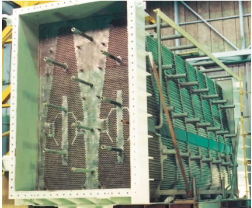
CM/H condenser module during fabrication, here ready for mounting of the water box cover 5
