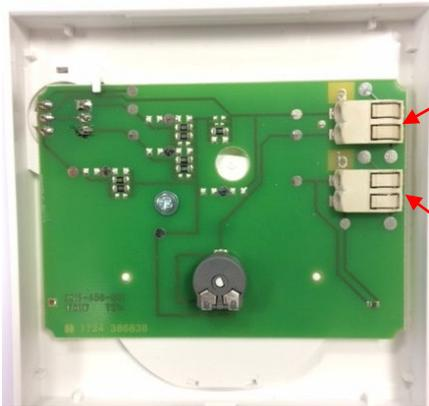
**Terminal a:** Output of the room control unit. This must be connected to “Input a” of the FCC. **(Setpoint adjustment)**
