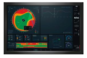
dow for the heli-operation based on the OCTOPUS response forecast. In this window the most optimal heading and maximum allowable motions can be selected to ensure a safe heli-operation.
