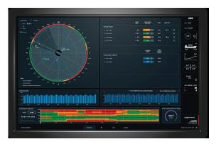
monitoring set-up provides unlimited amount of signals that can be monitored and provides dynamic KPI (key performance index) targets which can be used to follow the performance of the vessel subsystems.
