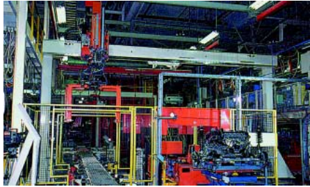
Transfer of engine packages in the automotive final assembly using an IRB 8400/ZP-6HD
