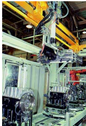
Assembly and handling of diesel engines using an IRB 8400/FP-5
