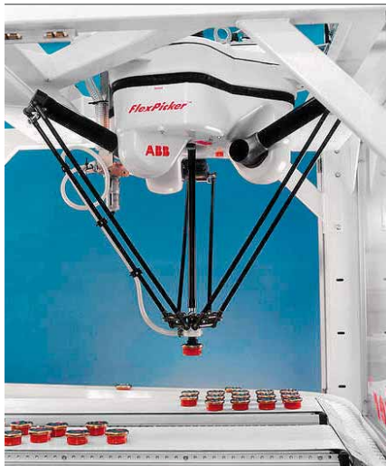
2 IRB 340, a parallel arm design
