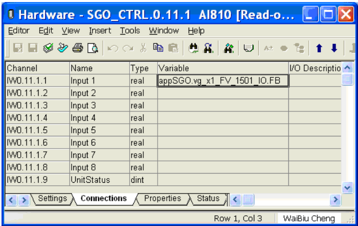
Figure 12. Insertion of Subvariable FB in an I/O Card
