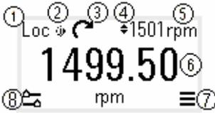
The screenshot shows a control panel with a speedometer reading 1499.50 rpm. It includes icons for local control, rotation direction, and menu options, numbered 1 through 8.
