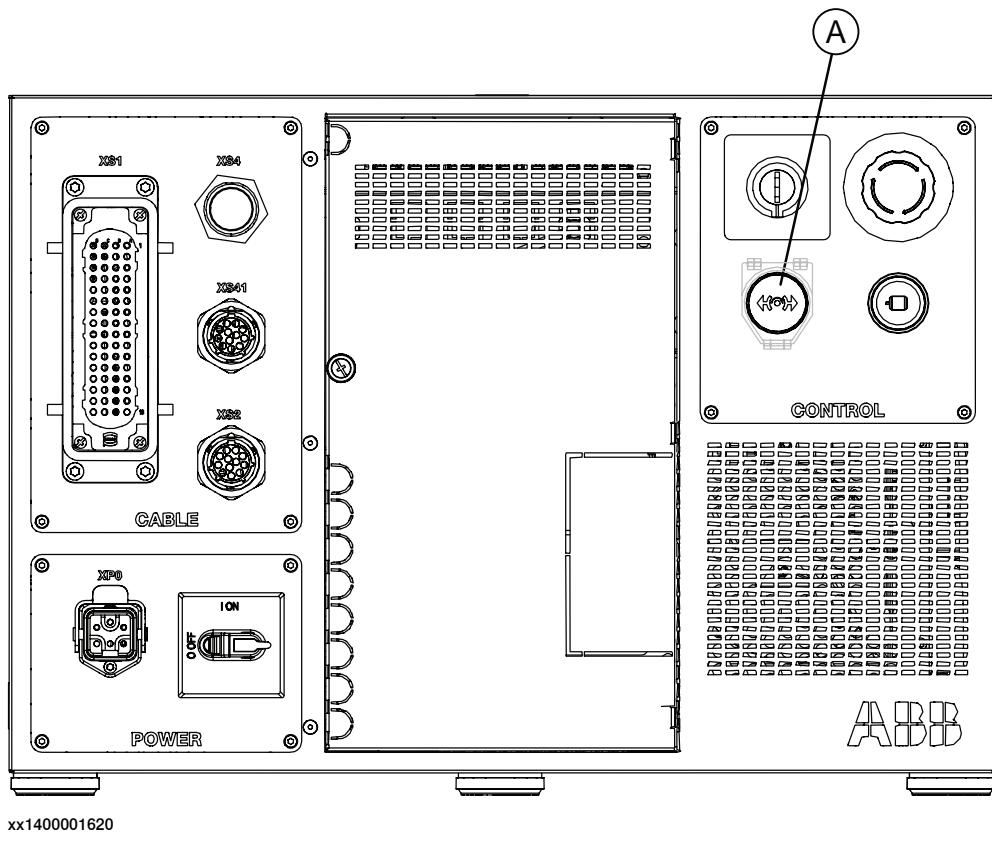
A      Brake release button (under the cover) for IRB 120.
