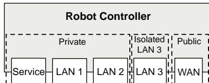
An alternative configuration is that LAN 3 is part of the private network. The ports Service, LAN 1, LAN 2, and LAN 3 then belong to the same network and act just as different ports on the same switch. This is configured by changing the system parameter *Interface*, in topic *Communication* and type *Static VLAN*, from "LAN 3" to "LAN". See *Technical reference manual - System parameters*.
