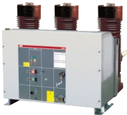
Fixed HD4 36 kV circuit-breaker with 350 mm pole centre distance: I_r = 630-1250-1600 A; I_{sc} = 16-20 kA.
