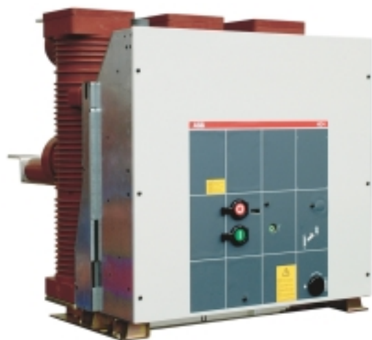
Fixed HD4 36 kV circuit-breaker with 275 mm pole centre distance: – I_r = 1250-1600 A; I_{sc} = 25-31.5 kA. – I_r = 2000-2500 A; I_{sc} = 20-25-31.5 kA
