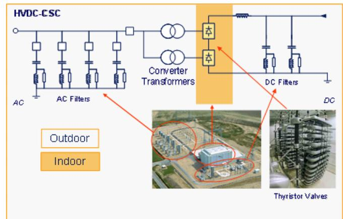
Figure 1 HVDC station with current source converters
