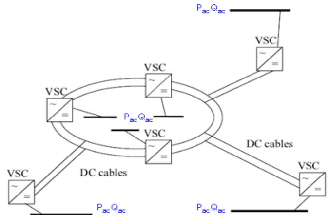
Figure 5 DC network embedded in existing city grid
