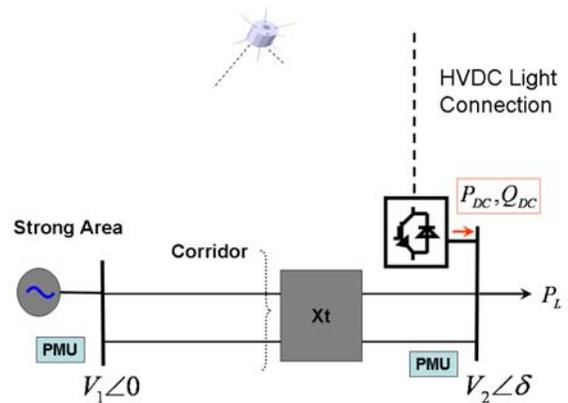
Figure 9 WAMS enabled control for maximum loadability
