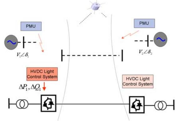
Figure 8 WAMS enabled control for oscillation damping
