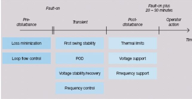
Figure 6 Application control functions of VSC-HVDC
