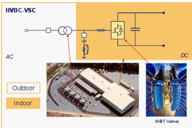
Figure 2 HVDC Station with voltage source converters
