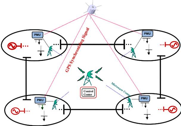
Figure 7 A wide area measurement system
