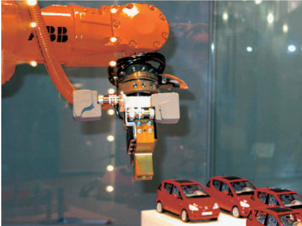
7 Wireless proximity switches on a robot gripper. Demonstration at Hanover Fair 2002
