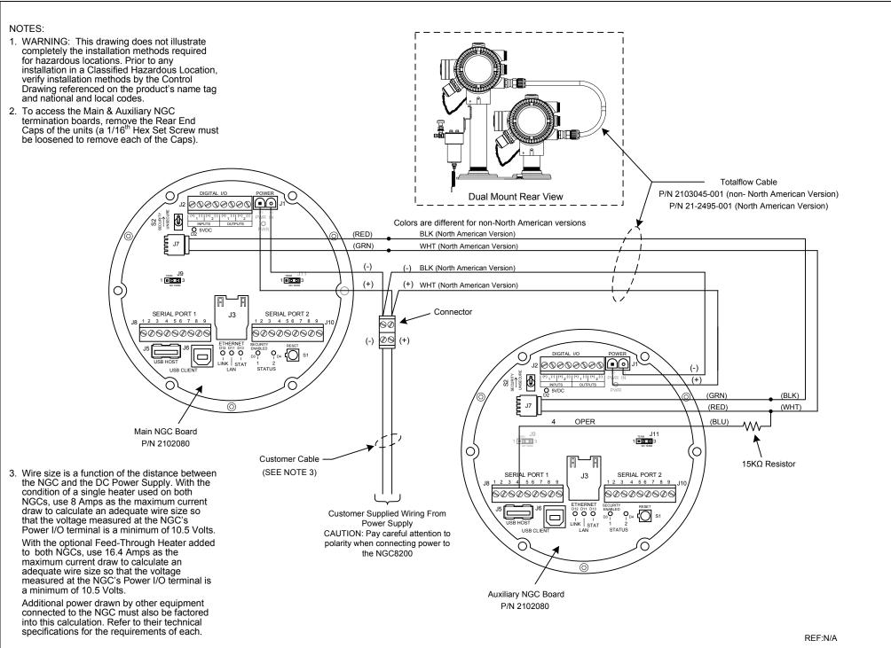
TOTALFLOW Products D20579 UD SHEET NGC DUAL8200 POWER AND COMM WIRING; MAIN UNIT TO AUXILIARY UNIT 2103087 AB 1 of 1
