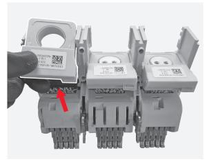
By means of the flat screwdriver lift the moving contacts assembly until it's unhooked from the lower case.
