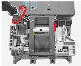
By means the cross screwdriver, unscrew the 2 screws located in the bottom part of the operating mechanism front cover fixing the operating mechanism cover to the circuit breaker main structure.
