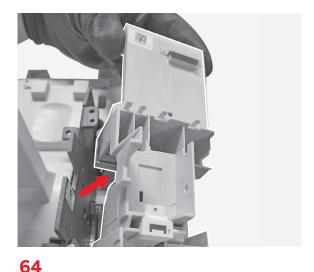
Manually remove the SY lever mounted on the left side of the operating mechanism.
