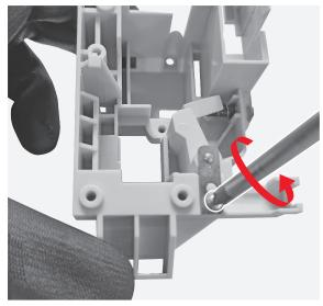
Manually remove the block lever.
