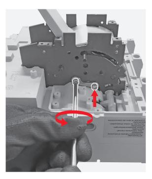
By means of the flat screwdriver push the shaft support as indicated by the arrow.
