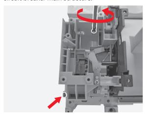
Manually pull the left base group as indicated by the arrow and after complete the removal.
