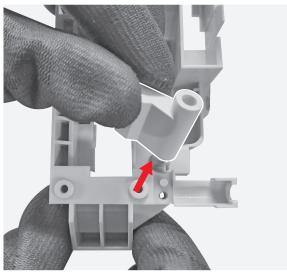
Manually remove the pin.
