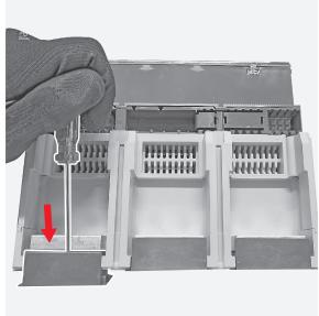
**5** By means of the flat screwdriver remove the nuts mounted on the cap kits.
