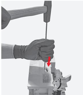
Put the circuit breaker with front up and push the rod as indicated by the arrow until the pin comes out from the hole left by the cover cap on the right side of the circuit breaker and after remove the rod.
