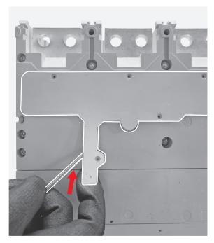
Manually remove the rear plate mounted on the lower part of the circuit breaker.
