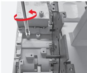
**66**Manually remove the wires cover and the wiring.
