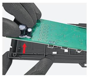
**34**By means of the pliers remove the "i TEST" pushbutton from the trip unit case.
