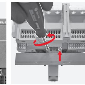
Manually push the cables protection as indicated by the arrow and remove it.
