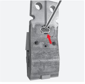
By means of the cross screwdriver unscrew the 2 screws fixing the fixed contact protection to the upper fixed contact and manually complete the removal operation.
