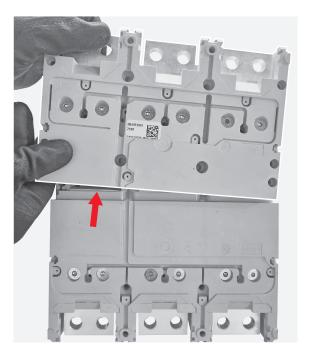
By means of the torx key (size 25) unscrew the 2 screws located in the back part of the circuit breaker.
