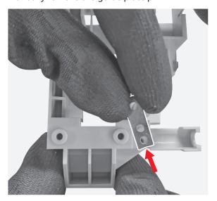
Manually remove the pin.
