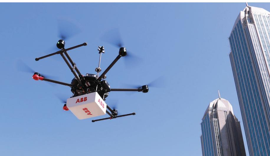
HoverGuard detects natural gas leaks around hard-to-reach sites such as bridges, high-rise buildings, areas with right-of-way restrictions or vegetation coverage, and pipelines.
