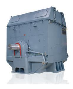
The stator core is built of stacked, high-grade, low-loss laminated electric sheet steel, insulated on both sides with a heat-resistant inorganic coating. Radial cooling ducts ensure uniform and effective cooling of the stator.
