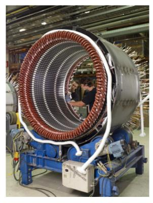
Form wound coils are used for medium or high voltage stators (also available for low voltage stators). High voltage coils include a semiconducting layer to decrease the electrical field at the slot surface.
