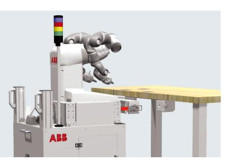
The YuMi docking station makes YuMi mobile and allows the quick and precise connection to an assembly station.
