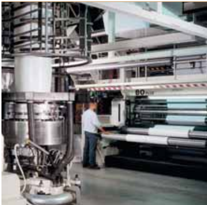
An Ideaplast plant in Italy with a single-line extruder (detail of the extruder's head and winding film rolls)
