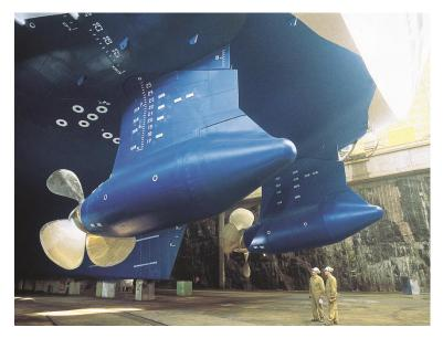
A typical ship propulsion system involves a massive arrangement consisting of a prime mover or generator (a diesel engine, gas turbine, etc.), power transmission equipment (a long and heavy shaftline with gearbox), steering and control systems, and finally, the propeller to provide motion. Much of the world's fleet uses some form of this diesel-mechanical propulsion system.
