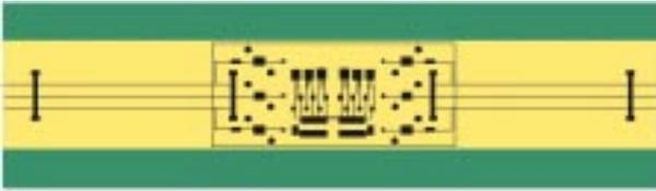
Figure 9 Modular back-to-back, overview. Fits in the right-of-way width of most AC lines.
