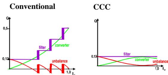
Figure 3 Reactive power conditions for a typical conventional converter and for a CCC.
