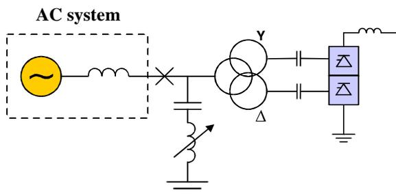
Figure 2 Single line diagram of a monopolar station with CCC and ConTune™ AC filter.
