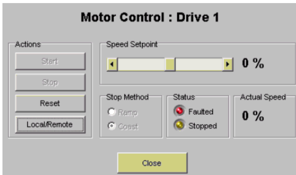
Figure 27. Motor control applet – drive faulted
