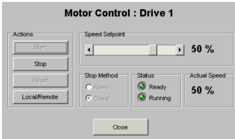
Figure 26. Motor control applet – drive running
