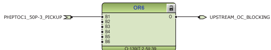
Figure 15: Upstream blocking logic
