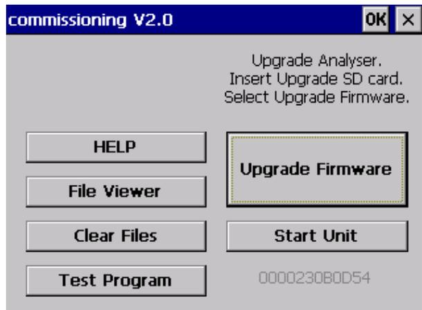
10. To upgrade the existing system software, press the **↵** key to start the process. (The software is transferred to the analyzer in sections.)
