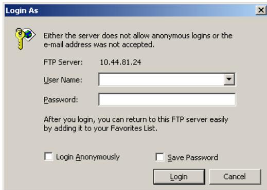
3. Type the 'User name' and 'Password' and press enter. The folders that are present on the analyzer are displayed.
