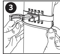
**Step 3: (optional):** For non-cylindrical surfaces TyRap® cable ties are recommended for additional fixation. TyRap® cable ties can be mounted above and below the Velcro™, following the "teeth" of the BCCH holder base.
