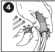
**Step 4:** Clip first half-shell of BCSR strain relief ring on terminal conduit (i.e., first wave trough of corrugated pipe). Press second half-shell tightly on top of first one until it "clicks" on both sides.
