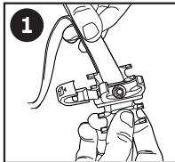
**Step 1:** Guide Velcro™ strap through one of the slits of the BCCH holder, starting on the inner surface of the BCCH holder base. Fold strap end around the base and press the rough strap surfaces tightly towards each other.
