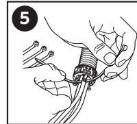
**Step 5:** To relieve strain on cables & tubes, fasten them individually to the "teeth" of the BCSR strain relief using TyRap® cable ties.
