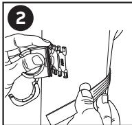
**Step 2:** Use the other side of the Velcro™ to fasten the BCCH holder tightly around the cobot arm.
