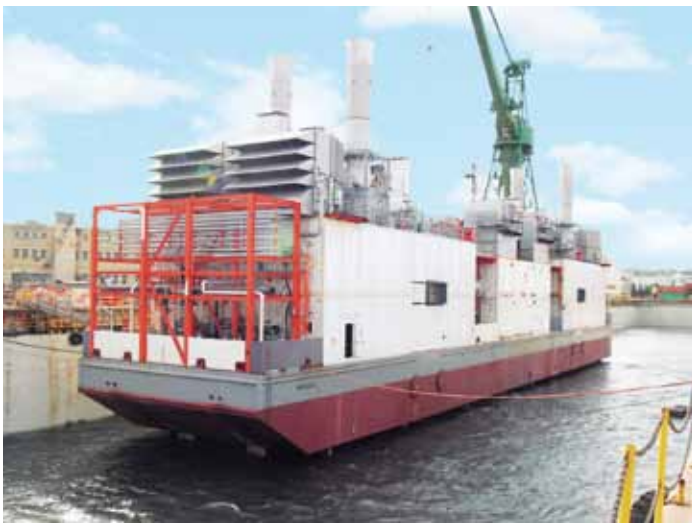
Power Generation Barge – 120 MW, Kazakhstan for Agip KCO
