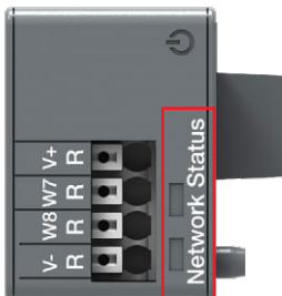
Fig. 5.17 Signals of Ekip Com DeviceNet -module
