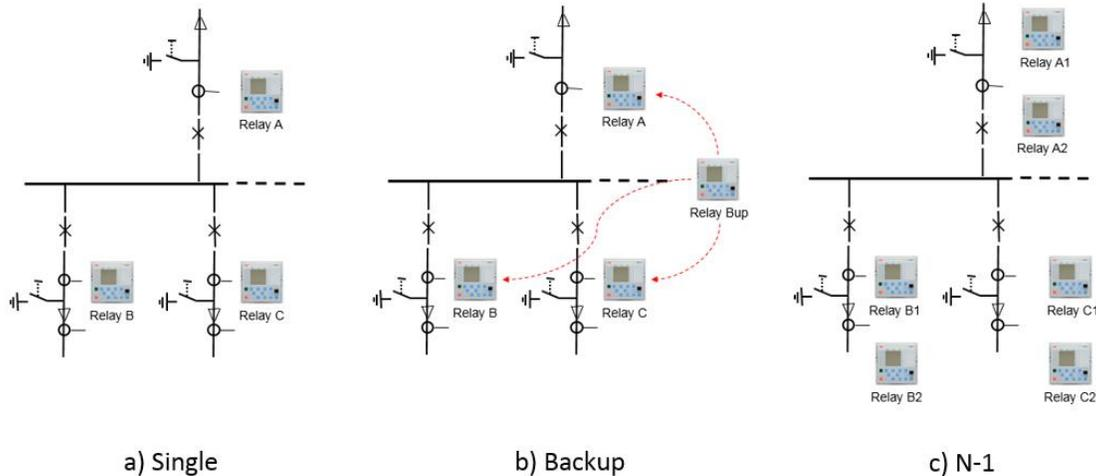
**Fig. 3** Three arrangements for multifunction bay protection relays in a decentralized secondary substation system: a) one relay per bay; b) one relay per bay and a “cold” backup relay for the entire substation; and c) redundant protection per bay.
