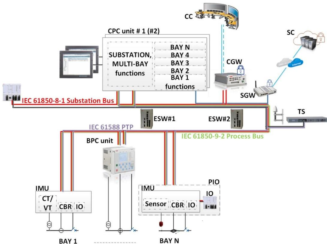
**Fig. 1** Hybrid protection and control secondary system architecture. Intelligent merging units and relays (BPC unit) are located at the bay level while the centralized protection and control (CPC) units are located at the station level.
