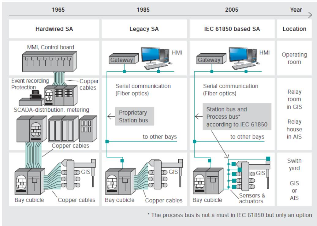
**Fig. 2** Secondary substation system in the three levels (process, bay and station levels from bottom to top) in three different stages: hardwired, Legacy and IEC 61850-based systems [7].
