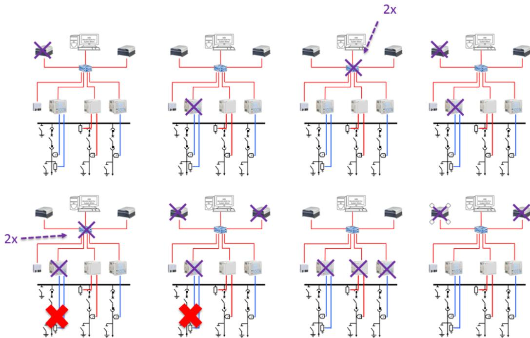
**Fig. 4** Eight failure scenarios (clockwise from top-left): one CPC unit out; one bay relay/IMU out; two Ethernet switches out (double failure); one CPC unit and one relay/IMU out; two CPC units out; three relays/IMUs out; two CPC units and one relay/IMU out; and two Ethernet switches and one relay/IMU out. In the latter two scenarios, one feeder (crossed in red) will be left unattended and protection from adjacent bays must be able to protect this feeder.
