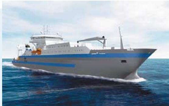
TyCom Reliance , Cable Layer 2 x 3.1 MW Propulsion Drives 2 x 3.1 MW Thruster Drives
