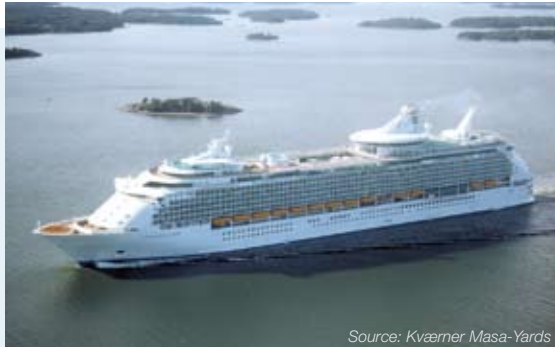
Navigator of the Seas , Cruise Liner 3 x 14 MW Propulsion Drives (ACS 6000c)
