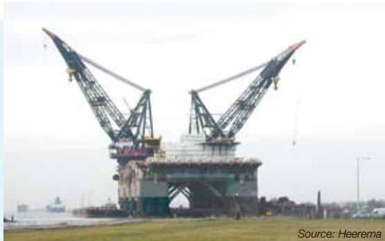
Thialf, Crane Ship 6 x 5.5 MW Thruster Drives (ACS 6000)
