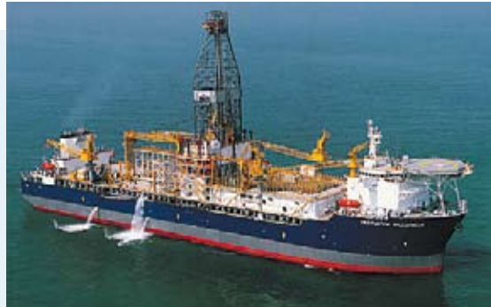
Deepwater Millennium , Drilling Vessel 6 x 4 MW Propulsion Drives
