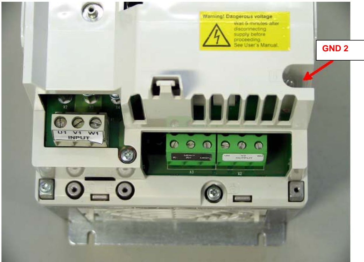
Figure 3: Earthing screw GND2 of the EMC capacitors in ACS800-01/U1 frame size R3.
