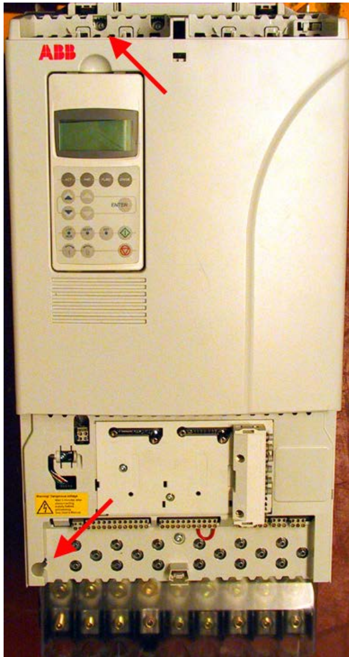
Figure 6.1: RFI earthing screws in frame R6.
