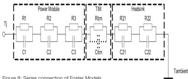
Figure 8: Series connection of Foster Models
