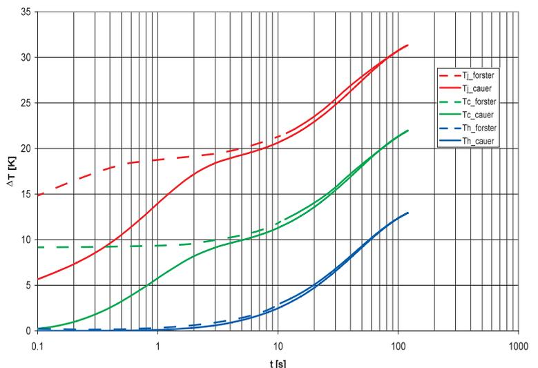
Figure 9: Temperature response of series connected models
