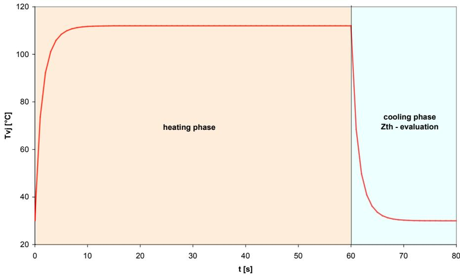
Figure 2 Temperature profile during Z<sub>th</sub> Measurement
