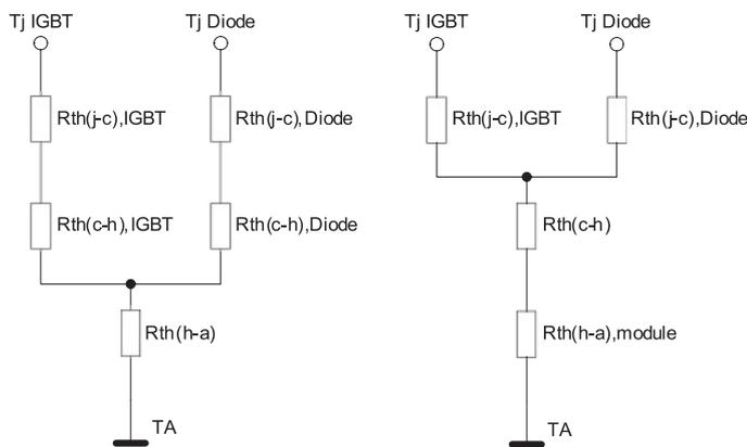
Figure 11: Modelling of the thermal interface
