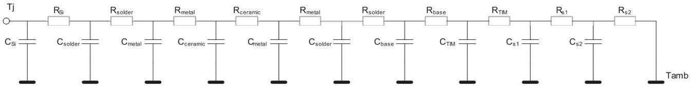
Figure 10: Series connection of Cauer Models
