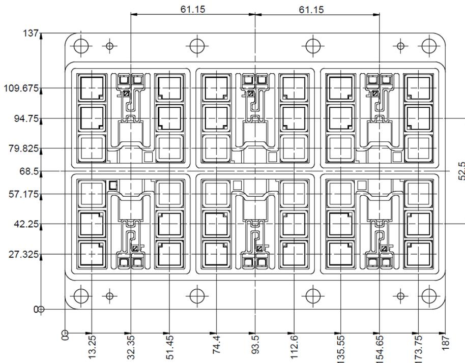
Figure 3: Chip Positions in a HiPak2 type module
