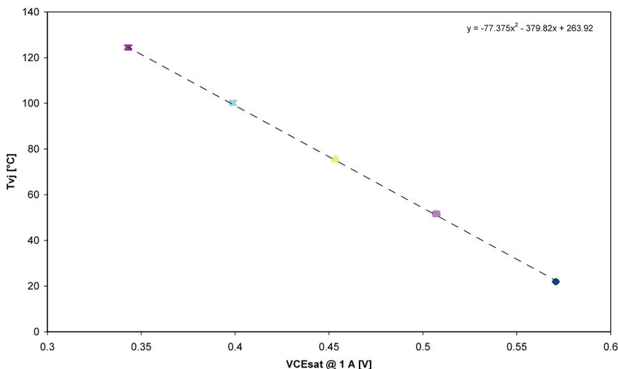
Figure 1: Calibration Curve  $V_{CEsat} = f(T_{vj})$
