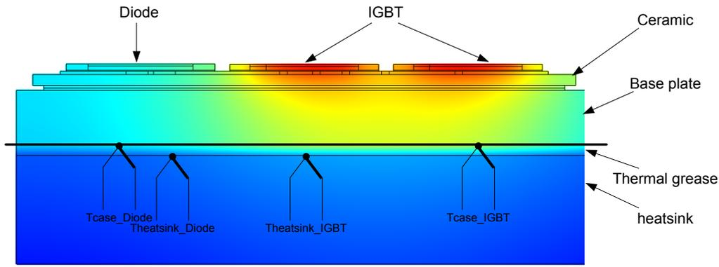
Figure 4: Location of case-temperature-probes
