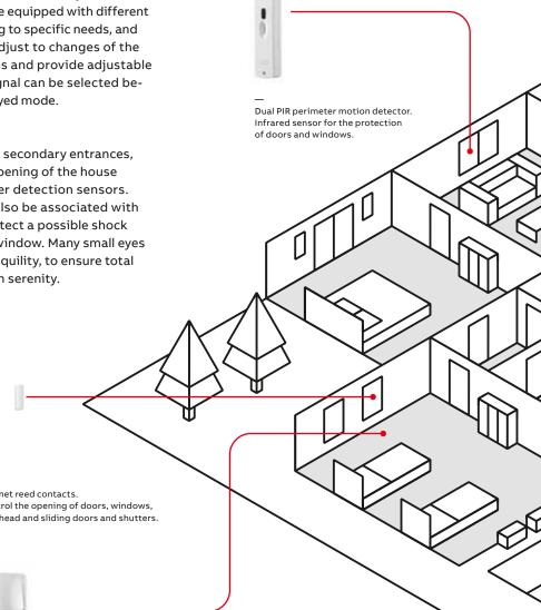
Magnet reed contacts. Control the opening of doors, windows, overhead and sliding doors and shutters.
