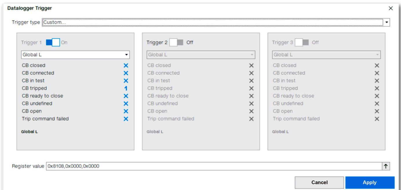
Figure 3 Trigger available inside the tool
