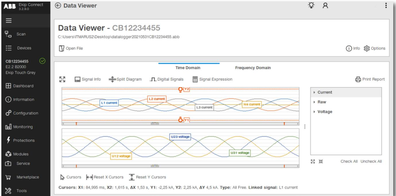
Figure 10 Graphical representation of split diagram function
