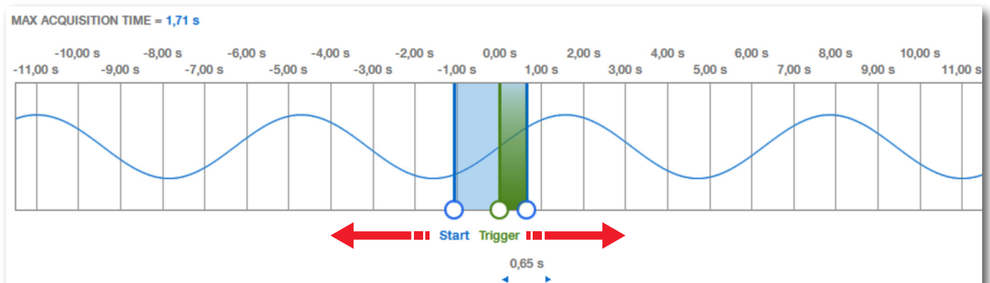
Figure 5 Time window that can be moved according to what I want to record before and after the trigger
