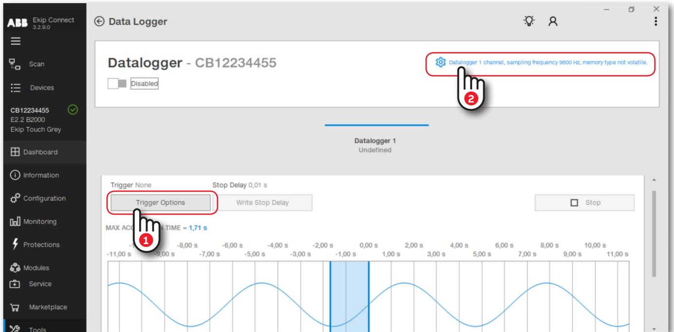
Figure 2 Datalogger tool inside Ekip Connect 3
